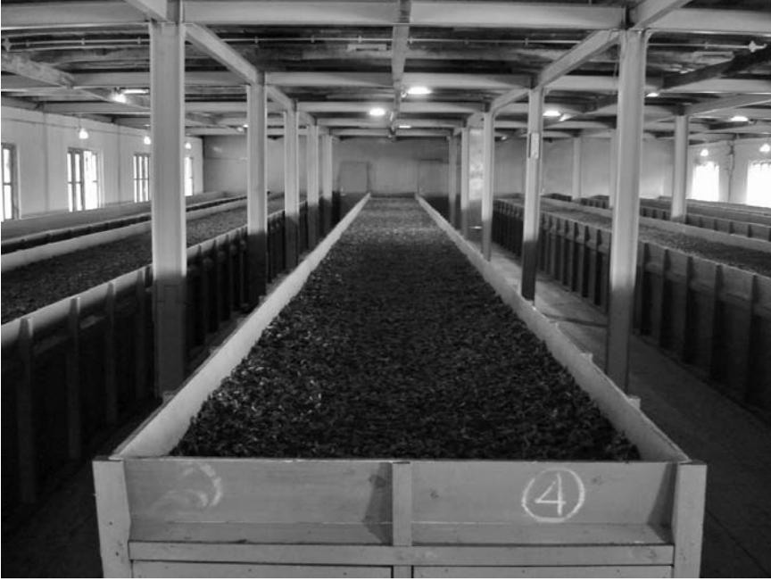
FIGURE 4. Tea withering in specially designed troughs in a tea factory. The process of withering removes the excess moisture from the tea leaves. Photo by author.
